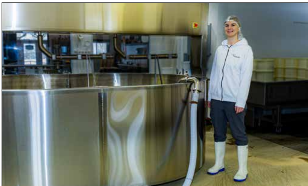
This tank holds the pasteurized milk and with added cultures and fermentation additives and produces the cheese's distinctive flavor as the milk becomes curds.
