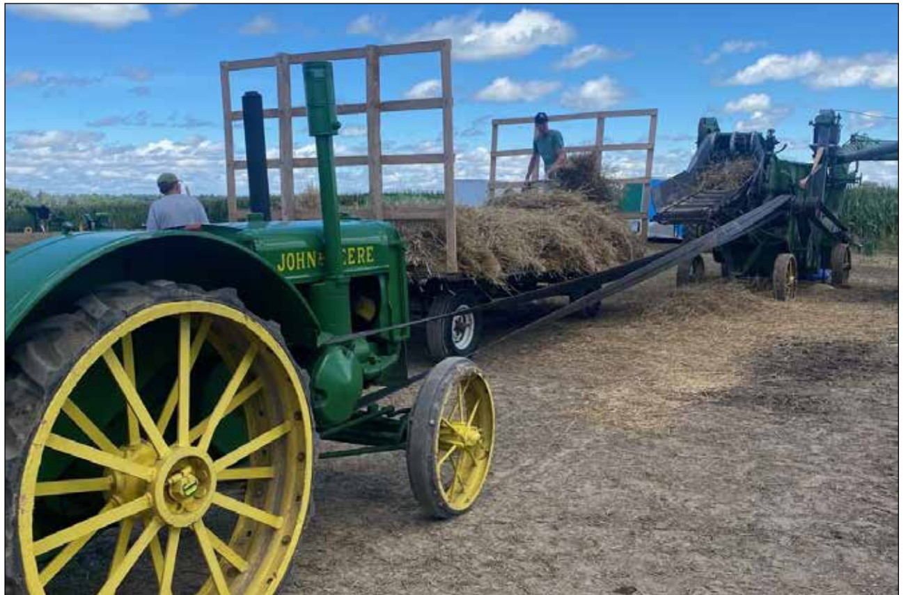
A threshing machine demo forking grain sheaves into the feeder of a John Deere threshing machine owned by Jared Buckrell of Burgessville and Brian Walton of the Hickson area. The tractor on the drive belt is a 1935 John Deere model "D", owned by Glen Garner, from east of Hickson.
