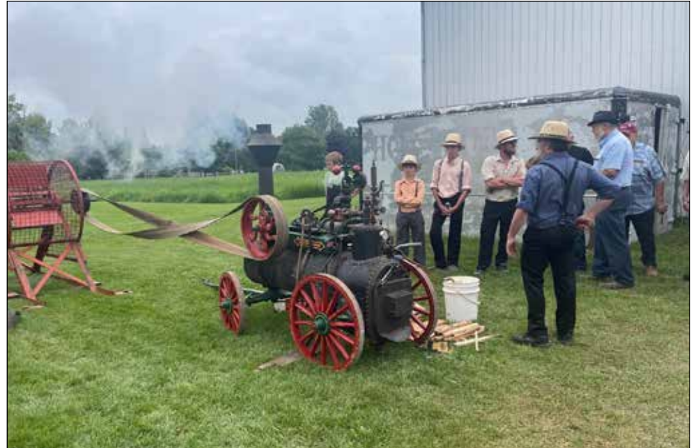
Many farmers who came to Gid Jantzi's last week, watched as neighbour Charles Walker demonstrated his drive belt powered Baker Fan, where the power came from his 1877 wood fired steam engine.
