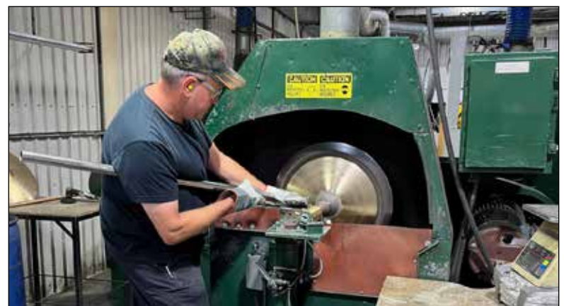
Polishing one of the 500 cymbals that will be produced on this particular day.
