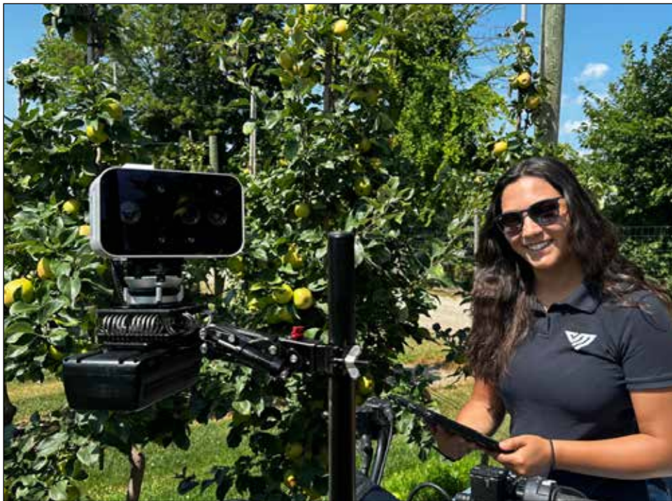
The Blue Mountain Fruit Company is utilizing a tool from Vivid Machines to perform rapid fruit counts and measurements of the trees in their orchard. The technology uses high tech cameras and machine learning.
