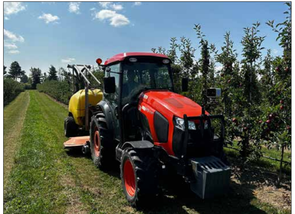
The Blue Mountain Fruit Company is utilizing a tool from Vivid Machines to perform rapid fruit counts and measurements of the trees in their orchard. The technology uses high tech cameras and machine learning.
