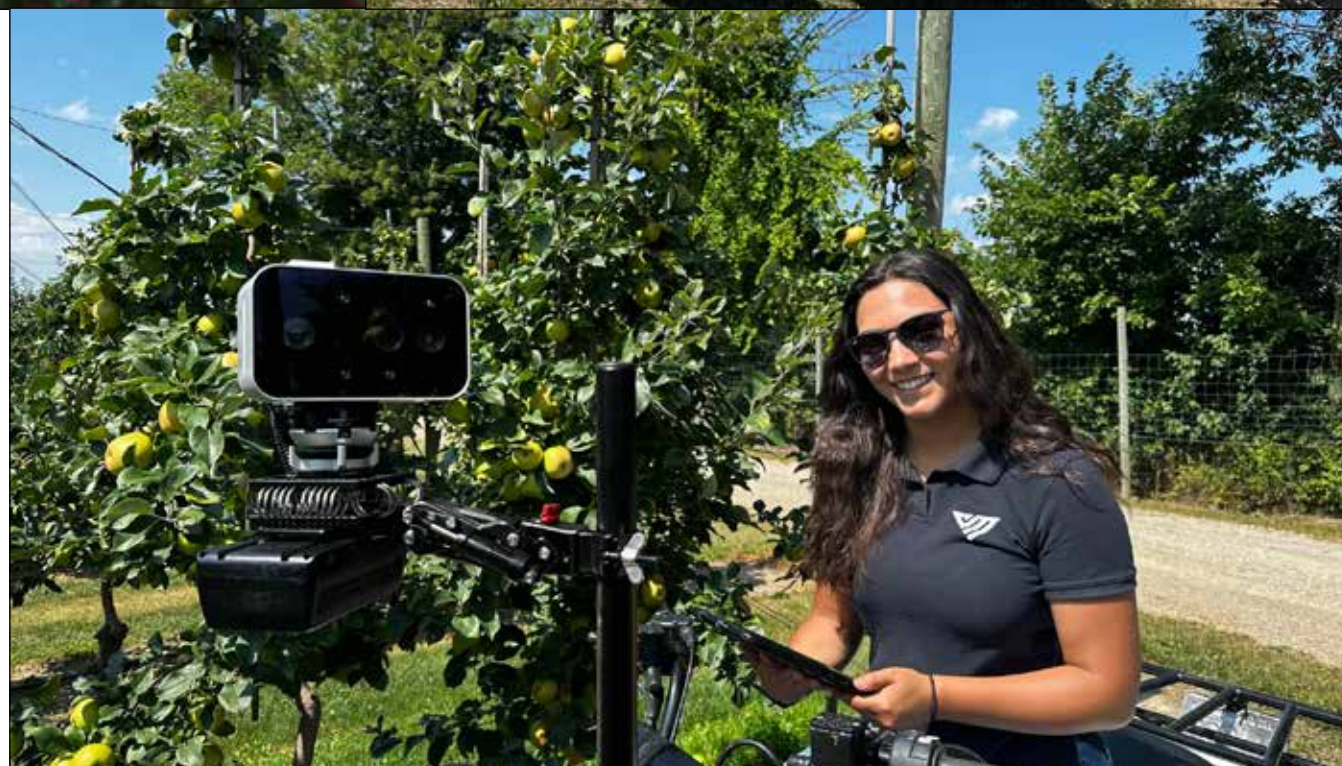
The Blue Mountain Fruit Company is utilizing a tool from Vivid Machines to perform rapid fruit counts and measurements of the trees in their orchard. The technology uses high tech cameras and machine learning. ~ Vivid Machines photos
