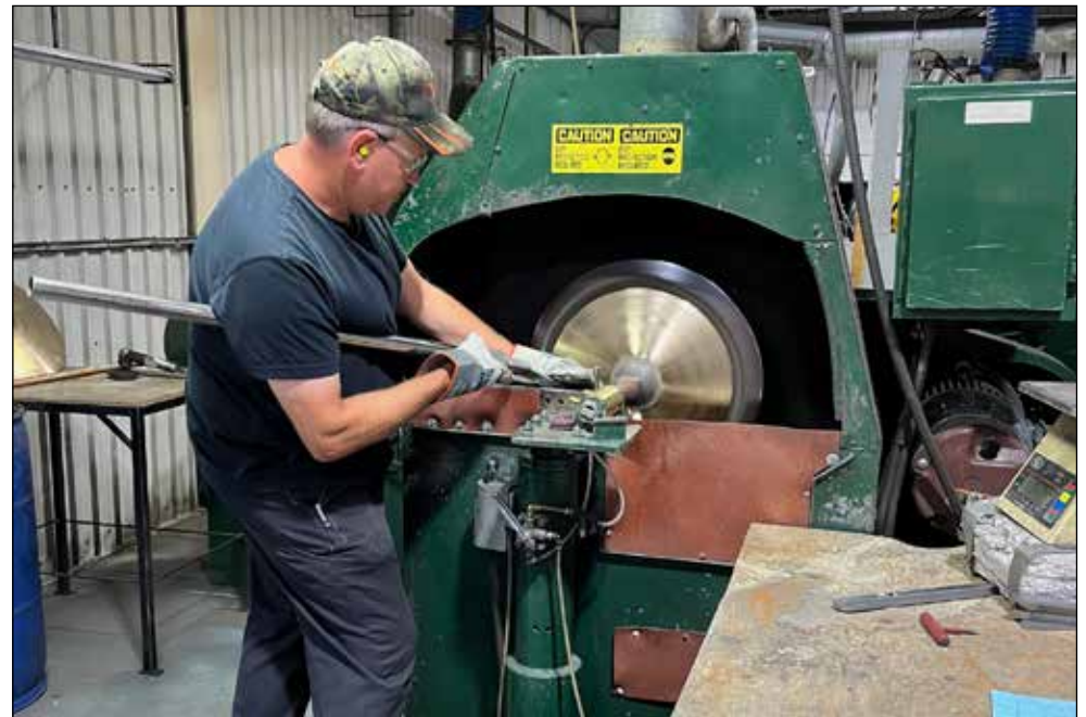
Polishing one of the 500 cymbals that will be produced on this particular day.
