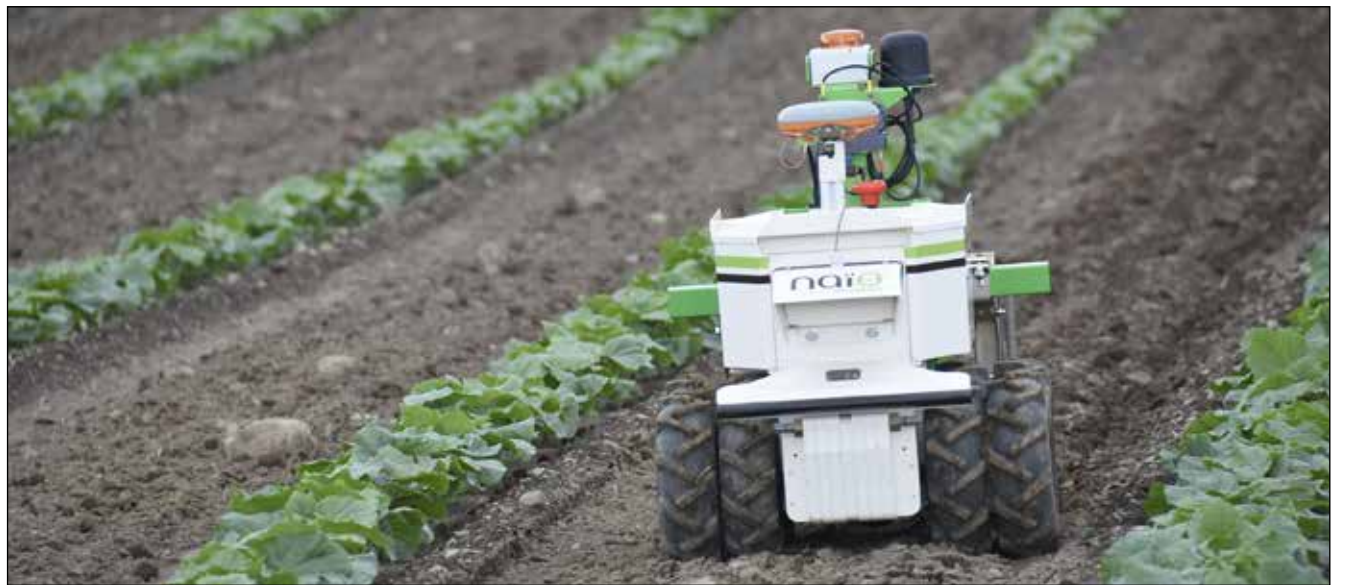
Naio Technologies Oz, a French-made electric tractor.
