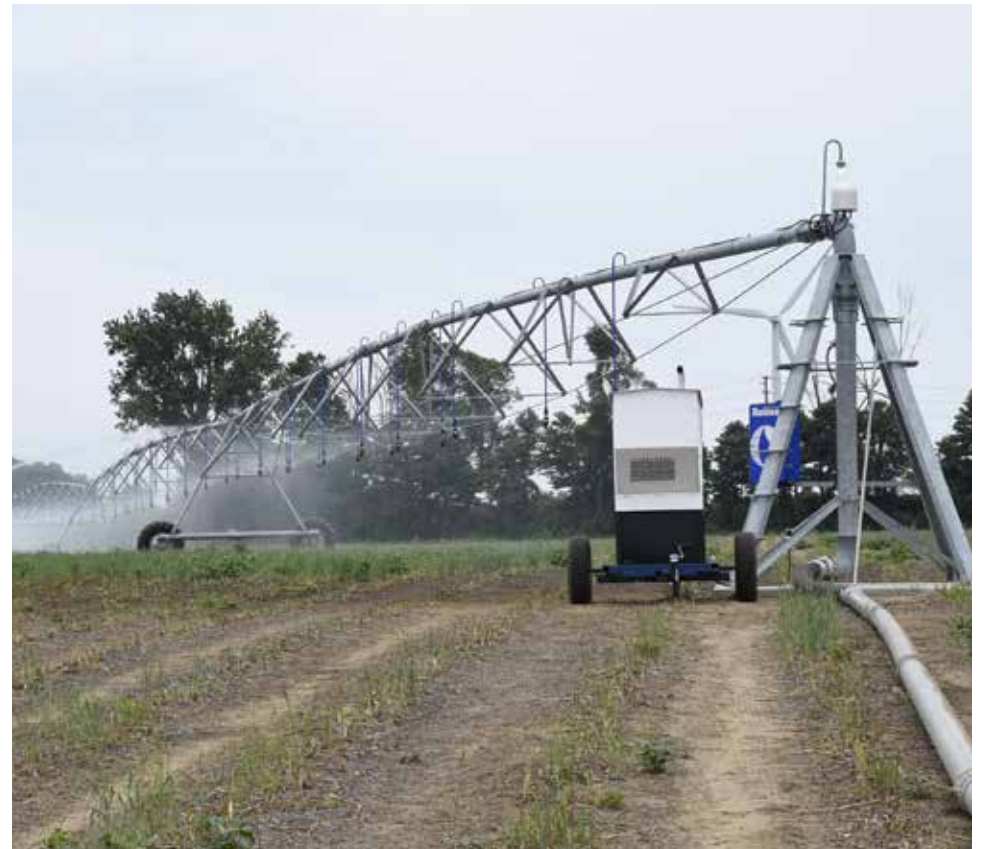
Pivot irrigation systems are more efficient than travelers and less work for the farmer as moving it is not needed.
