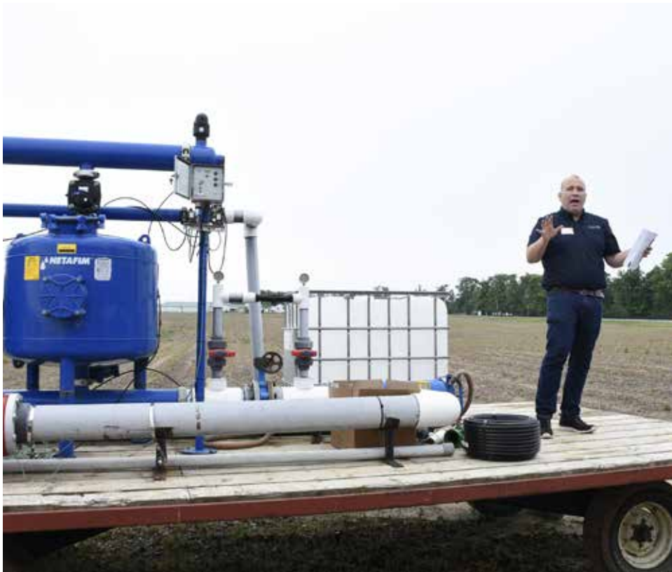
Philippe-Michael Caron of Dubois Agrinovation explained the merits of drip irrigation while standing next to a display showing the pumping unit, injector and other components for this irrigation type.
