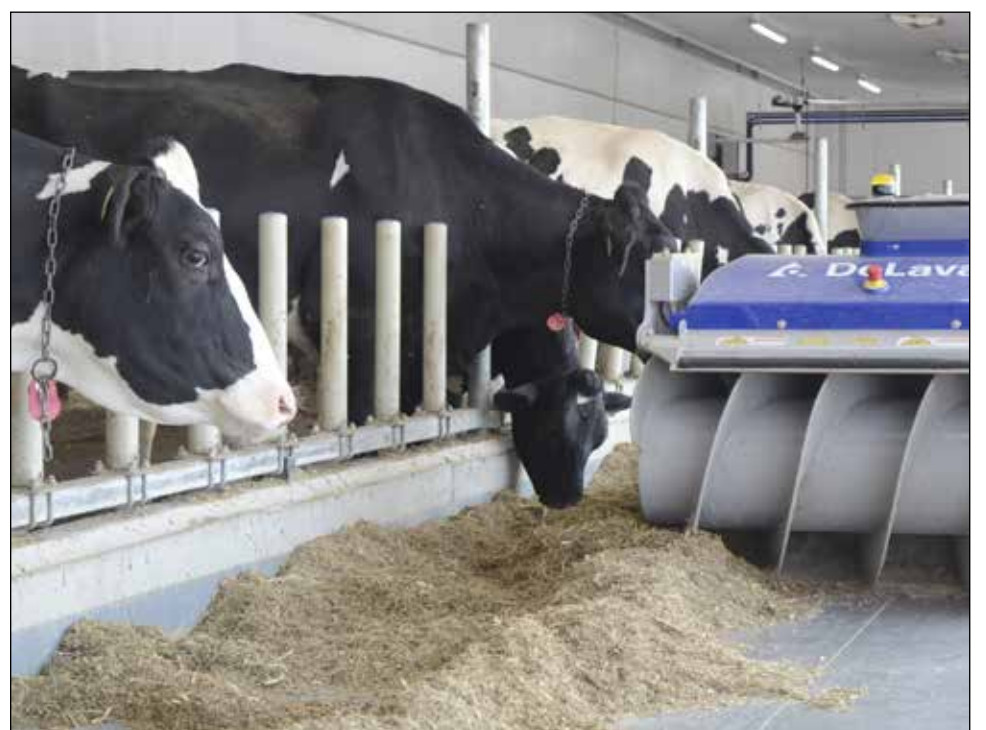
This OptiDuo feed refresher takes regular trips to make sure the feed is within reach of John DeBoer's cattle in his new robotic dairy barn in St. Anns.
