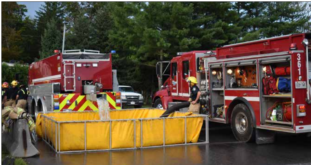
If there is no water source immediately available on a rural property, firefighters battling a blaze may use a portable water tank, like the one seen here, as an alternative source. The portable water tank would be constantly refilled by tanker trucks driving in a circuit from the nearest hydrant or other viable water source.
